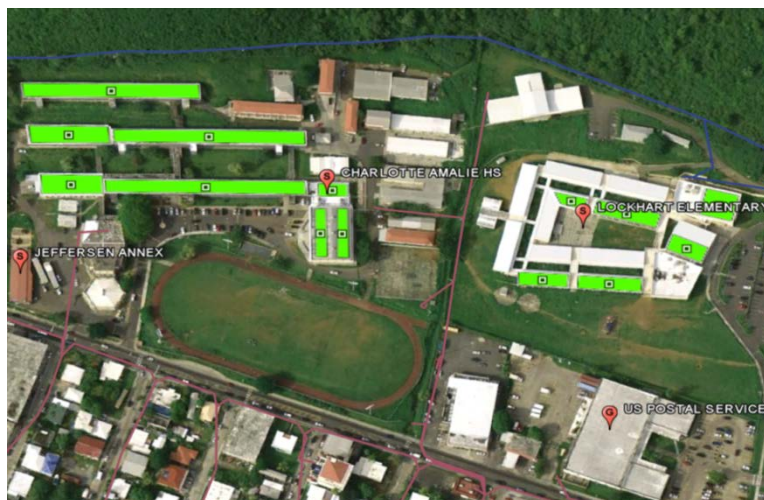
Figure 5-1. Roof area survey screen shot, St. Thomas, with potential PV locations identified in green
