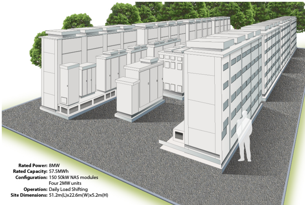
Figure C-4. Layout of 8-MW NaS battery system
