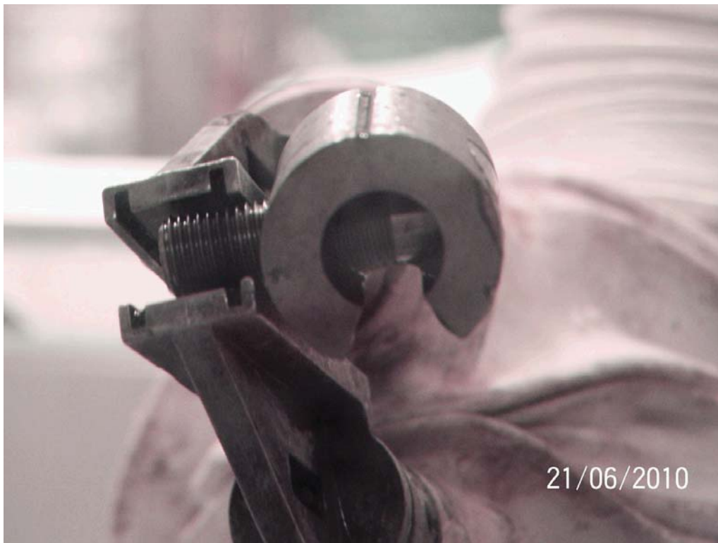
Figure 9. The One C-Ring that was Successfully Removed in Hot Cell 1E1.
