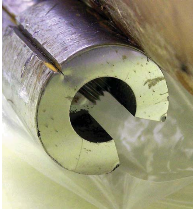
Figure 11. Pre-Stressed C-Ring VS-ENC-W (S10R000240) Showing Stress Bulge is Undisturbed.
