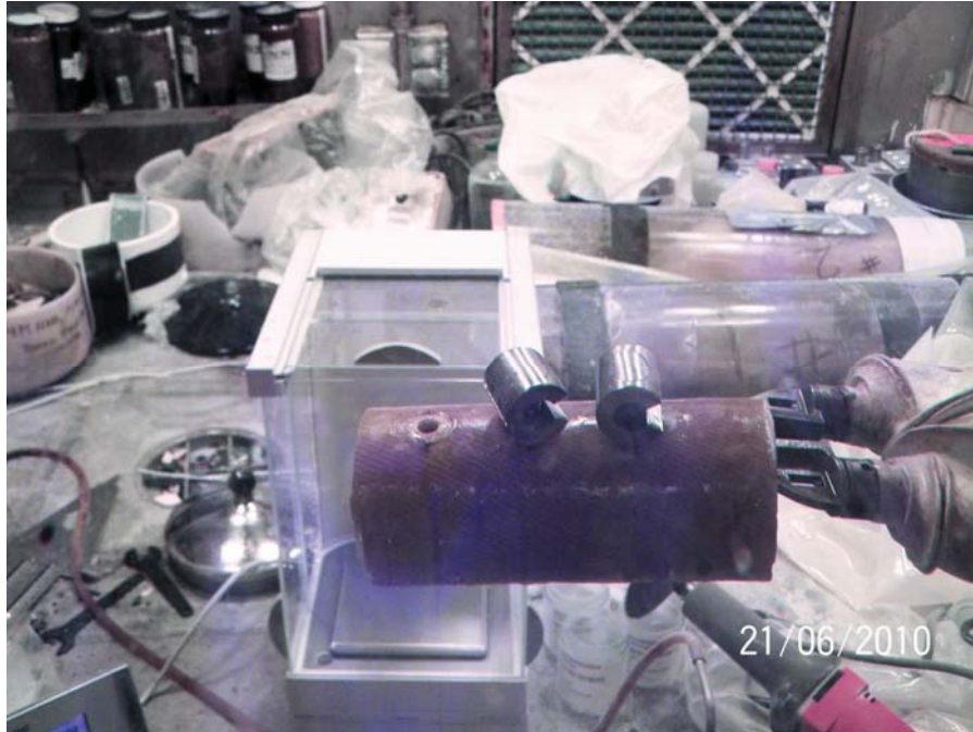
Figure 7. The Half-Foot Long Section of Detector 1 with 2 C-Rings Attached.
