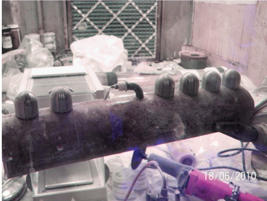
Figure 8. The Foot- Long Section of Detector 2 with the Supernatant Probe Section Bullets.
