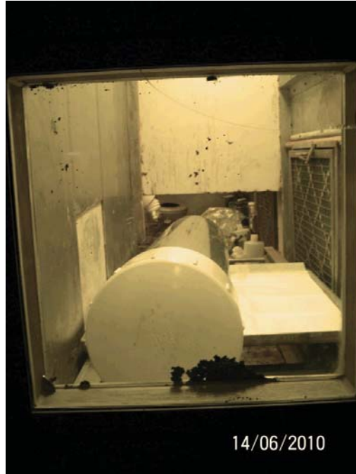
Figure 3. Detector Section 1 in Hot Cell Airlock.
