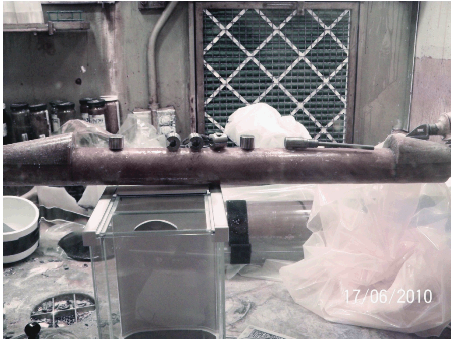
Figure 5. Detector Section 1, Unpackaged in Hot Cell 1E1.
