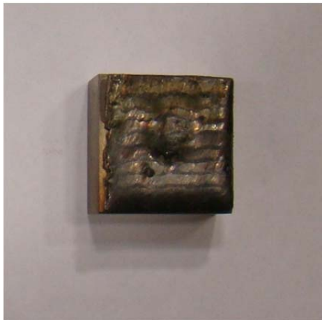
Fig 12. (a) Optical image of the Ni cladding processed on an Alloy 800H substrate using a laser power of 3500W. (b) Cross-sectional optical microscopy of sample shown in (a).
