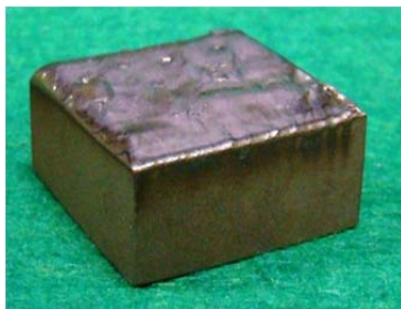
Fig 3. Optical image of a Ni-based alloy substrate with a Ni cladding applied using a laser-based surface cladding technique.
