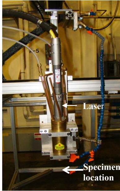
Fig 2. Image of the laser setup used for laser processing of claddings.
