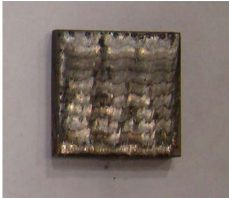
Fig 7. (a) Optical image of the Ni cladding processed on an Alloy 617 substrate using a laser power of 3000W. (b) Cross-sectional optical microscopy of sample shown in (a).
