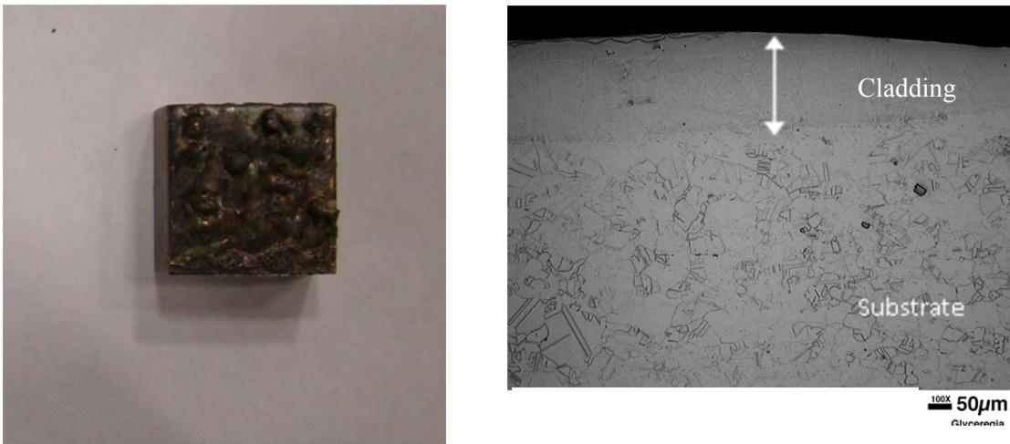
Fig 10. (a) Optical image of the Ni cladding processed on an Alloy 800H substrate using a laser power of 2500W. (b) Cross-sectional optical microscopy of sample shown in (a).
