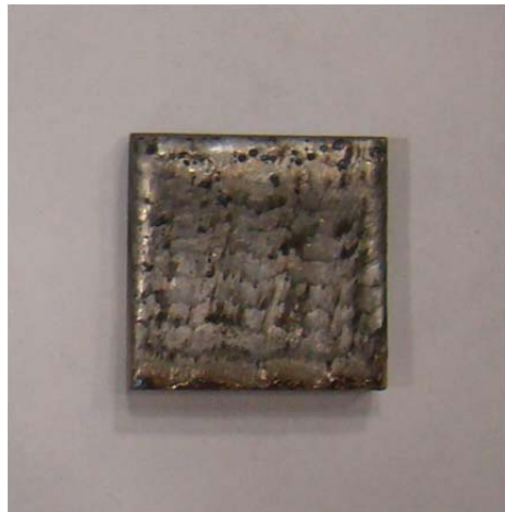
Fig 8. (a) Optical image of the Ni cladding processed on an Alloy 617 substrate using a laser power of 3500W. (b) Cross-sectional optical microscopy of sample shown in (a).
