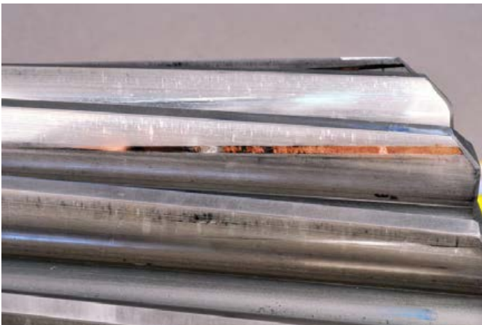
Sun Pinion (Severe Fretting Corrosion) Photo from GEARTECH, NREL/PIX 19750
