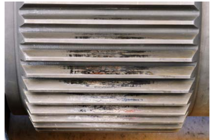
Sun Spline (Severe Fretting Corrosion) Photo from GEARTECH, NREL/PIX 19751
