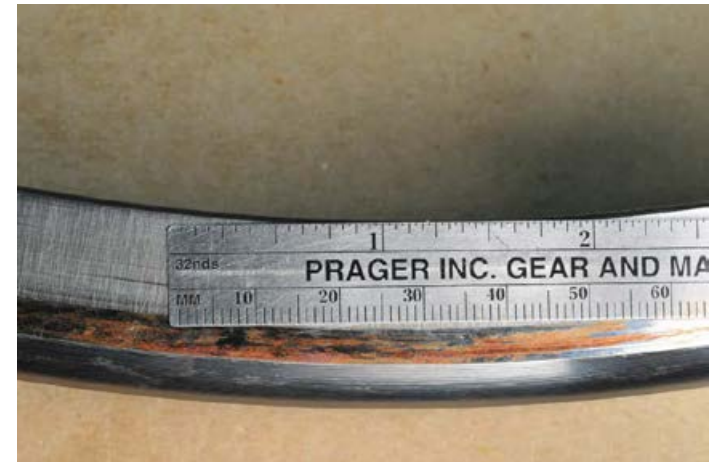
Bearing PLC-A Outer Raceway (Severe Fretting Corrosion) Photo from GEARTECH, NREL/PIX 19748
