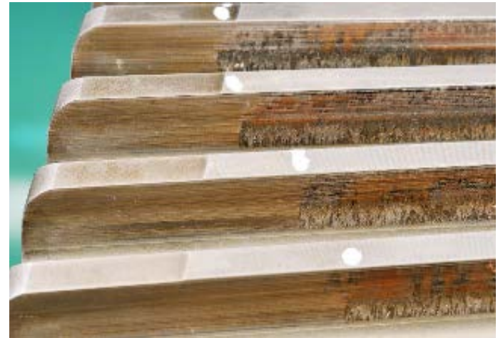
High-Speed Stage Gear (Severe Scuffing) Photo by Robert Errichello, NREL/PIX 19599
