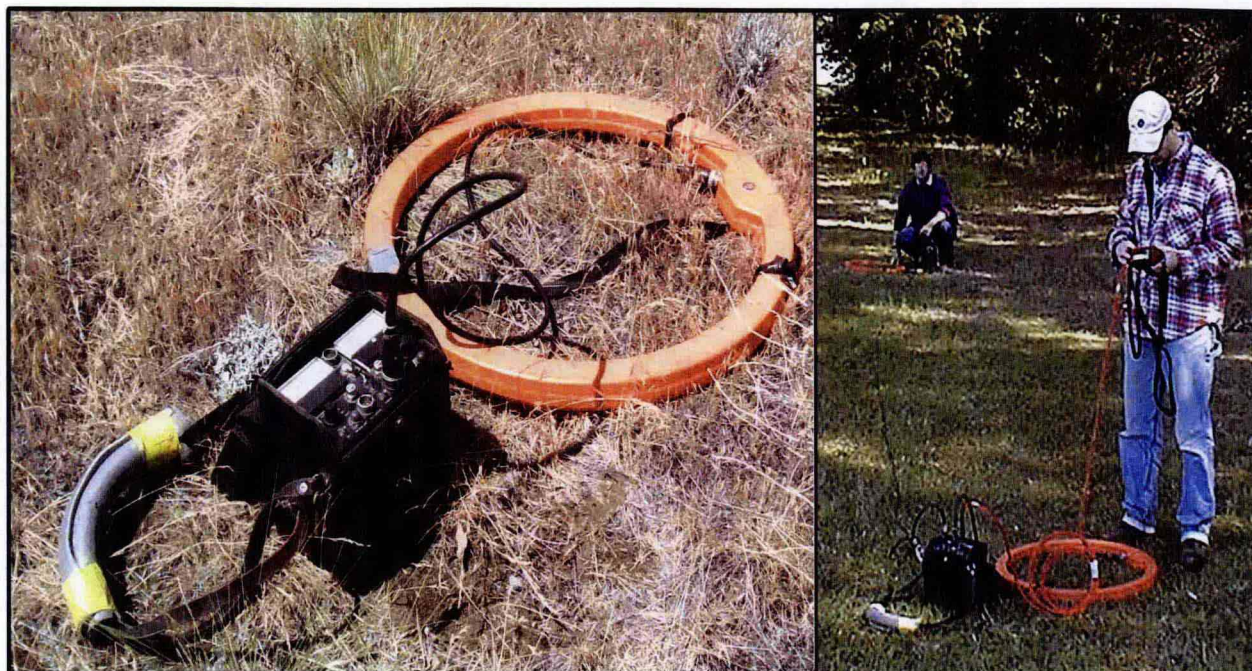
Figure A-8. Geonics EM-34 Instrument
