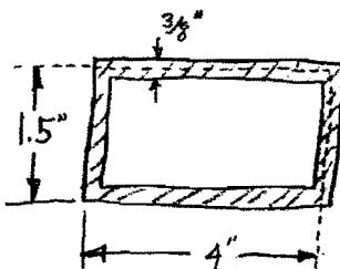
$$\begin{aligned} \text{Area} &= (1.5 + \frac{3}{16})(4 + \frac{3}{16}) \\ &\quad - (4 - \frac{9}{16})(1.5 - \frac{9}{16}) \\ &= 3.84 \text{ in}^2 \end{aligned}$$
