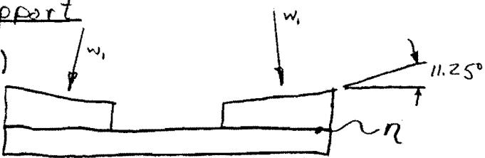
The only support holding the blocks (horizontally) is friction.
