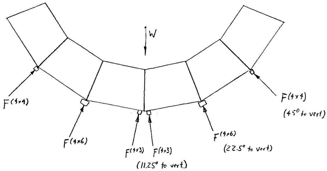
This shows positioning of the strap beams on the OH assembly
