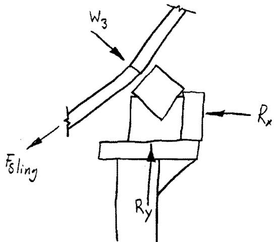
The force  $F_{\text{sling}}$  is neglected completely, making the estimate of  $R_x$  ( $W_{\text{max}}$ ) used on the next several pages very conservative.
