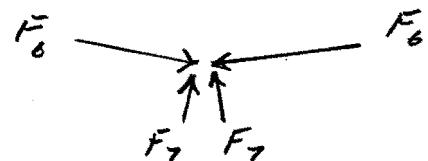
$$F_7 = F_6 \frac{\sin 22.5^\circ}{\cos 11.25^\circ} = (6702 \text{ LB}) \left( \frac{\sin 22.5^\circ}{\cos 11.25^\circ} \right) = 2615 \text{ LB}$$
