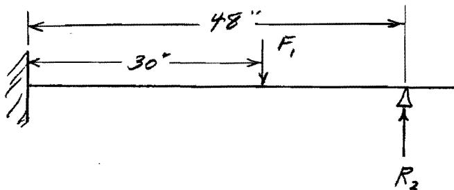
$$R_2 \text{ (from 180nm SPREAD SHEET)} = 1554 \text{ lb}$$
