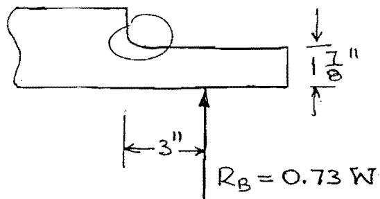
At notch at downstream end of cradle bar:
