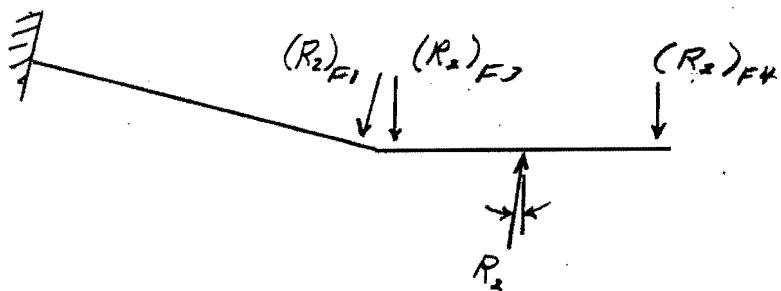
$$\sum F_y = (R_2)_{FJ} + (R_2)_{FK} + (R_2)_{F1} (\text{cos } 22.5^\circ) - R_2 (\text{cos } \theta) = 0$$
