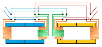
Figure 8: Schematic diagram of the connections for a pair of corrector dipoles mounted close to each other on the "blue" and "yellow" rings. The green windings are the compensation coils connected in series with the main coils of the opposite magnet.
