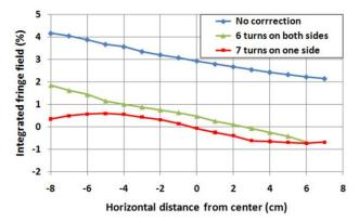
Figure 9: Results of tests performed to determine the best configuration of the coils used to compensate the cross-over field affecting the opposite ring.
