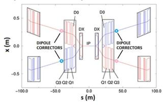
Figure 1: Schematic view of the RHIC "6 o'clock" interaction region. The circles indicate the approximate locations of the corrector magnets close to the cryostats.
