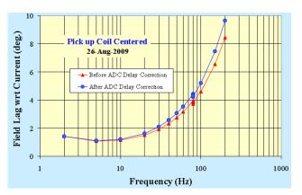
Figure 4: Measured frequency response of the prototype laminated yoke corrector magnet.
