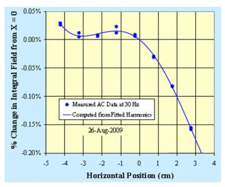
Figure 3: Example of measured integrated field variations as function of distance from the nominal beam axis, obtained with a 0.61 m long flat coil and 30 Hz field excitation in this case.
