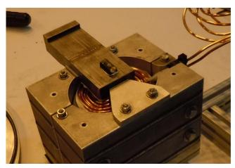
Figure 6: Coil in potting mold ready for vacuum impregnation.
