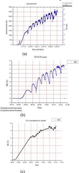
Figure1 GaAs photocathode activation. (a) is the yo-yo orocess with excess oxygen, ;(b) is the yoyo process with excess Cs; and, (c) is the saturation process
