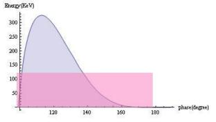
Figure 2 The energy of the electron backbombardment response to the RF phase of the photocathode. The x ray generated by electron backbombardment energy in the pink range cannot pass the Dewar's wall.
