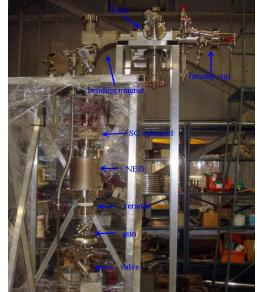
Figure3 Gun assembly in the beam line
