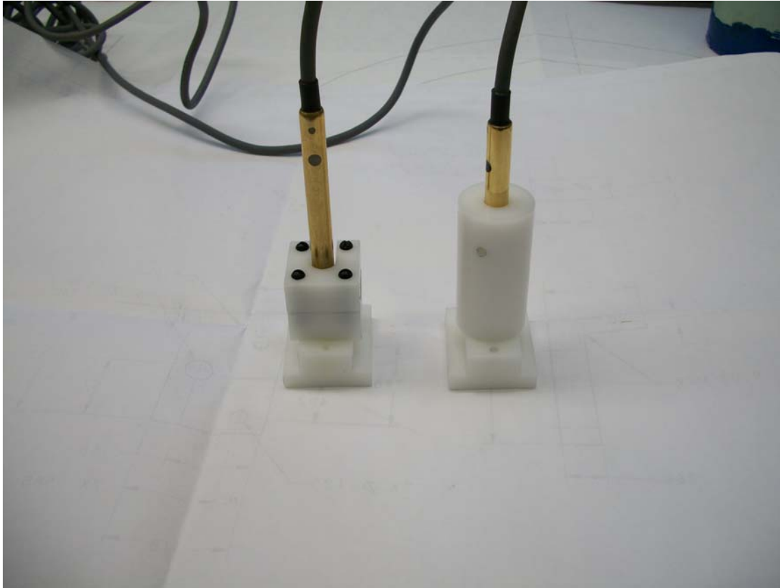
Fig 3.6. Transverse fluxgate probe (left) and axial fluxgate probe (right) in holders.
