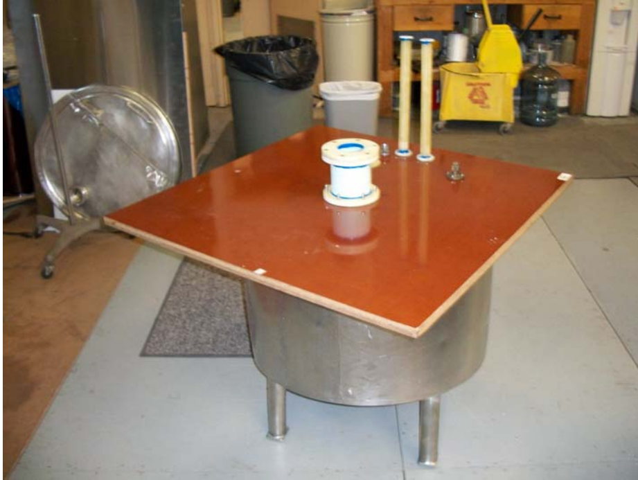
Fig. 3.3. Test cryostat with cover and warm bore tube.
