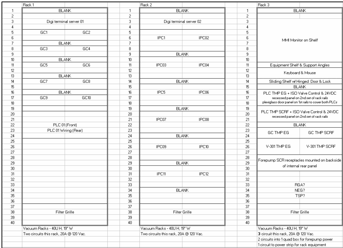
Figure 12. ERL Mezzanine Vacuum Instrumentation Control Rack Layout
