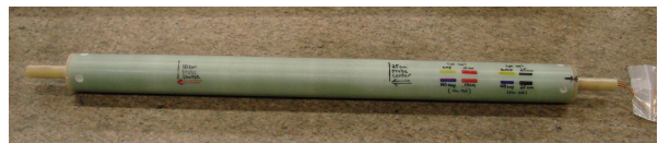
Figure 1: The circuit-board probe used in the measurement. The 100 mm coil is close to the left end.
