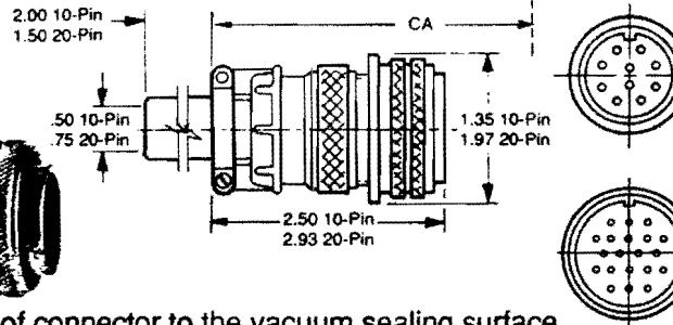
Note: CA (Connector Attached) is the distance from end of connector to the vacuum sealing surface.
