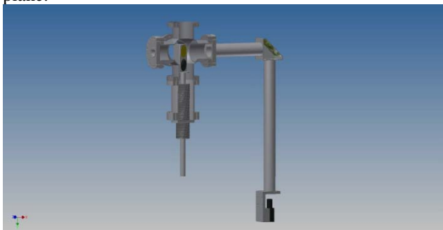
Figure 2: Conceptual design of the beam flag that will be produced by Radiabeam Technologies
