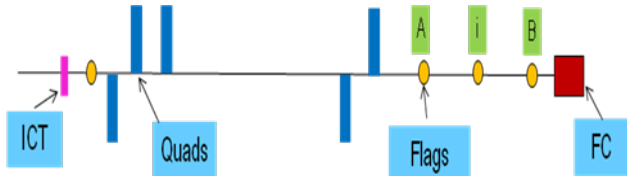
Figure 5: Layout of the transport line to the first dump. Beam enters from the left side.
