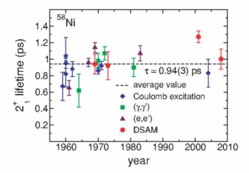
FIG. 5. (Color online) Average value obtained for the lifetime of the  $2_1^+$  state in <sup>58</sup>Ni. The average comprises twenty measurements, including this work, and gives a final standard value of  $\tau = 0.94(3)$  ps.
