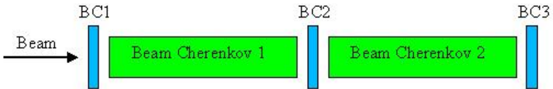
Figure 2.2: Beam Čerenkov detectors system layout
