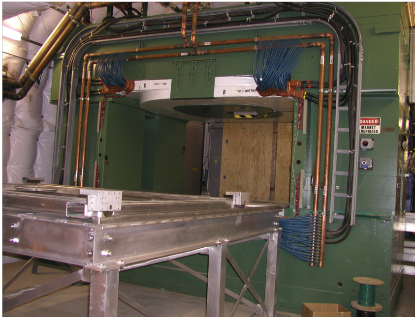
Figure 2.11: Jolly Green Giant analysis magnet creates 0.7 T magnetic field to bend charge particles inside the TPC volume.
