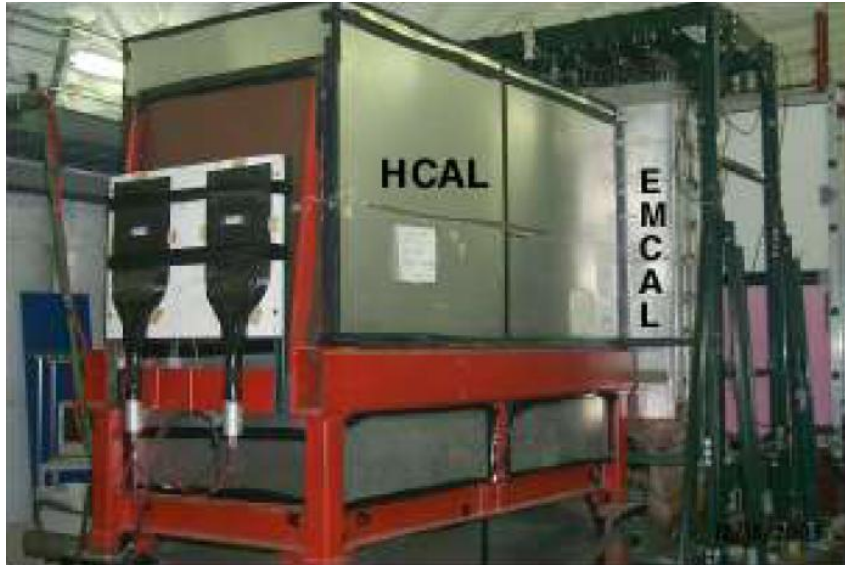
Figure 2.10: The MIPP calorimeters, HCAL and EMCAL were used for neutral particles.
