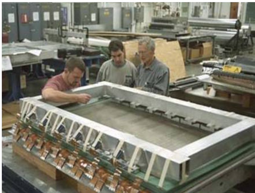
Figure 2.3: MIPP experimenters are working on one of the MIPP's drift chamber.
