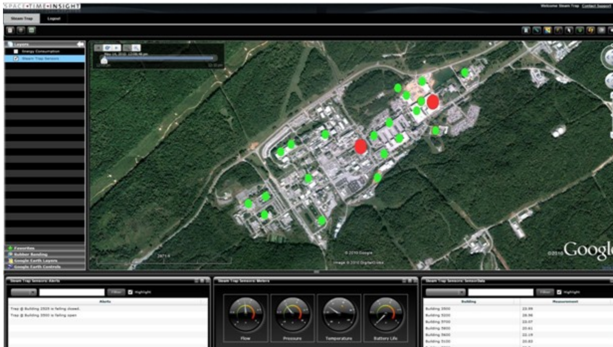
Fig. 9. The situational awareness interface used to visualize sensor data from the wireless sensors along with status alerts.
