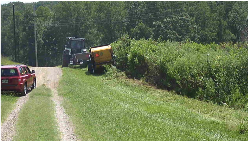
Figure 3. Sites #1 (above) and #2 of the BioBaler test harvest at the UT Arboretum on August 9th, 2011. These sites contained mostly herbaceous material and were not effectively baled.
