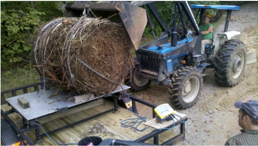
Figure 7. Weighing the bales on a portable digital scale. Tissue samples were taken from each bale for moisture content and proximate and ultimate analysis.
