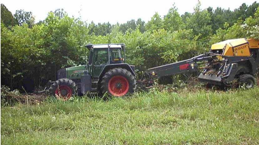
Figure 4. Site #3 (0.5"-4" woody vegetation) of the BioBaler test harvest at the UT Arboretum on August 9 th , 2011. This site was effectively baled.
