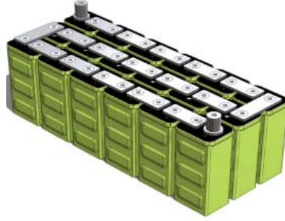
Fig 1 structure of supercapacitor module
