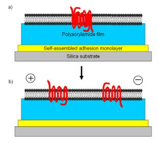
investigating two ways of improving electrophoretic mobility: better polymer supports, and a novel nanoporous medium that suspends the bilayer over free solution.
