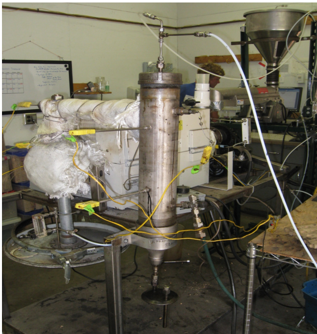
Figure 1.11. Setup of mixing column for biodiesel and biooil.
