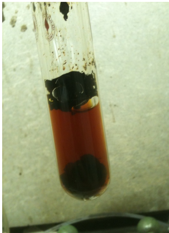
Figure 7.2. Solid disc formed over the hydrolysis products of ILC aqueous phase bio-oil and PCC catalyst.
