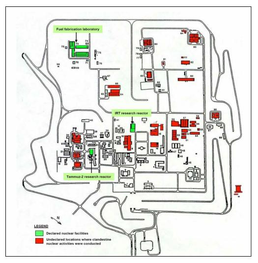
Fig, 1, In this schematic drawing of the Tuwaitha site, the buildings highlighted in green correspond to the declared facilities that were under IAEA safeguards, while buildings highlighted in red were used, exclusively or in part, for undeclared nuclear activities.<sup>8</sup>
