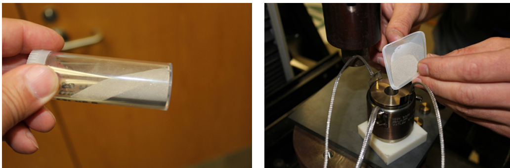
Figure 9. Dried silver powder (left) and it being poured into the mold (right).
