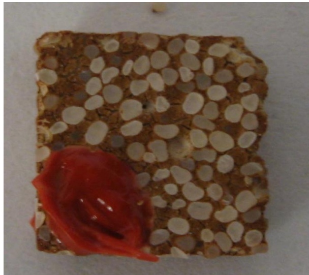
Figure 9.6. Photograph of Concrete Coupon after SPFT Experiment
