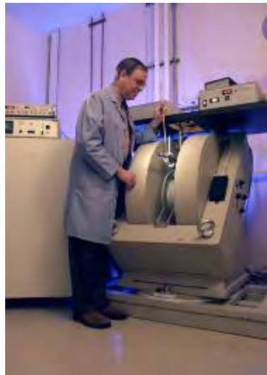
**Figure 11.** Bruker pulsed EPR/ENDOR/ELDOR spectrometer.
