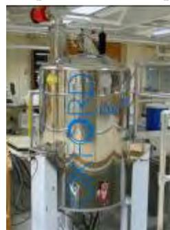
**Figure 3.** Varian INOVA 750-MHz NMR spectrometer.
