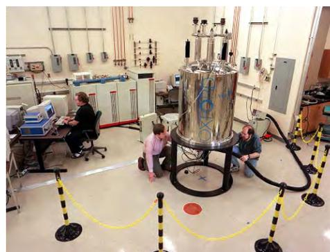
**Figure 6.** Varian NMR System 500-MHz wide-bore NMR spectrometer.
