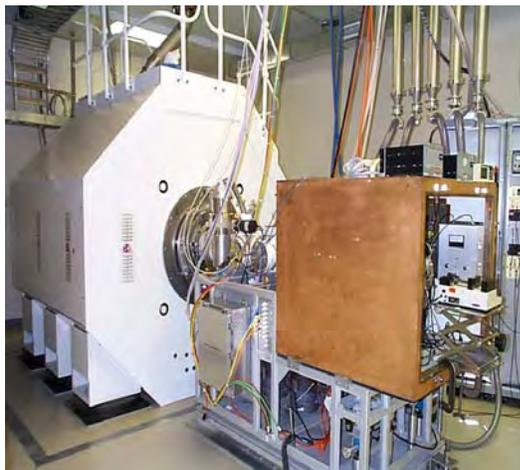
**Figure 2.** Wide-bore, passively shielded 11.5-T FTICR MS.
