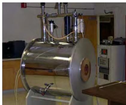
**Figure 10.** Horizontal-bore 2-T magnet.
