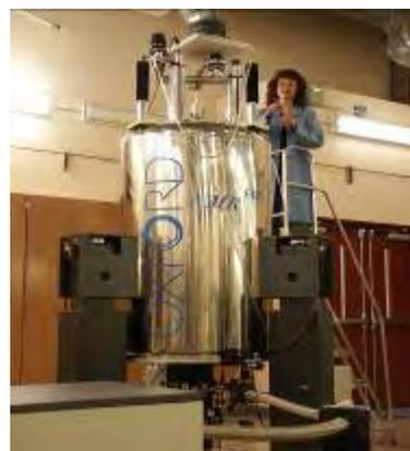
**Figure 4.** Varian INOVA 600- MHz NMR spectrometer with Cryoprobe.
