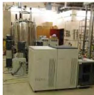
**Figure 5.** Varian INOVA 600-MHz NMR spectrometer.
