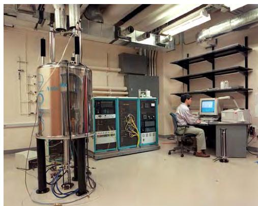
**Figure 9.** Varian/Chemagnetics Infinity 300-MHz NMR spectrometer.
