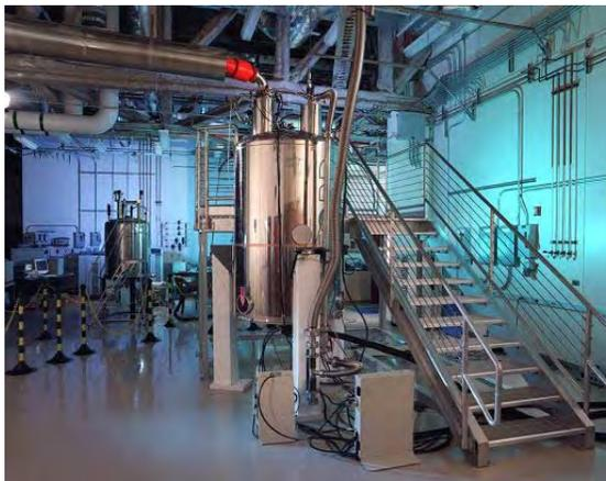
**Figure 2.** Varian INOVA 800-MHz NMR spectrometer.
