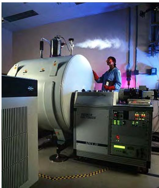
**Figure 3.** 150-mm-bore, actively shielded 9.4-T FTICR instrument.
