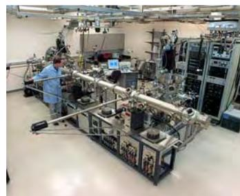
*Figure 1. Oxygen plasma-assisted MBE system.*
