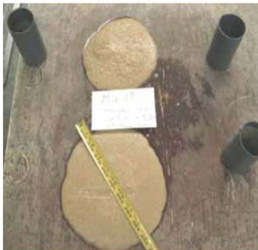
Figure 3-3. ASTM D-6103 Flow Test and example of self-leveling grout. Modified test used smaller (2 x 4 inch) cylinders.
