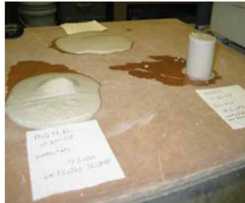
Figure 3-2. Visual observation of liquid phase segregation.
