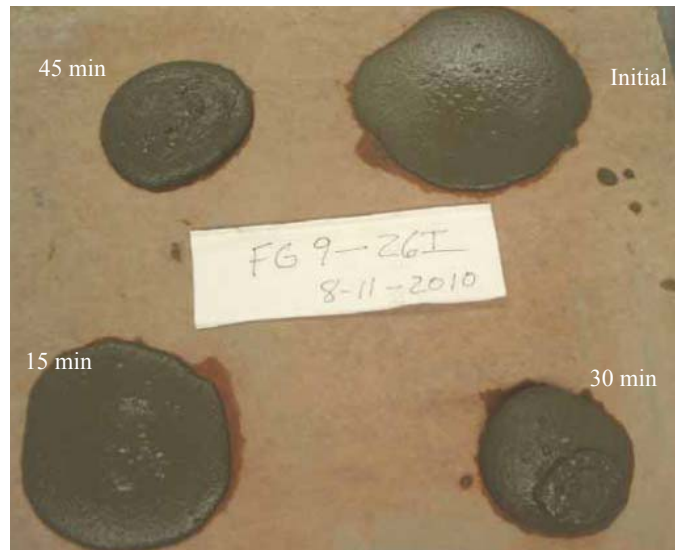
Figure 4-3. Static flow test results for Mix FG-26I (boric acid mix) per modified ASTM D-6103. Initial spread and spread after increasing times under static conditions.
