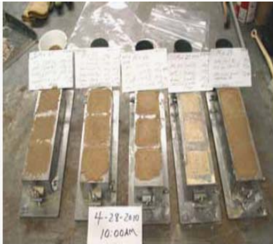
Figure 3-5. Compressive strength cubes prepared per ASTM C-942 prior to stripping molds.
