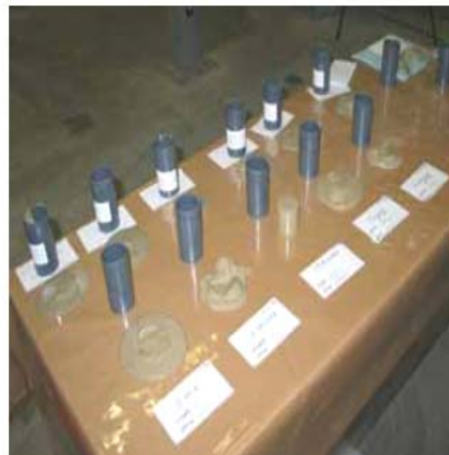
Figure 3-4. Static working time test samples. Modified after ASTM D-6103 by performing at selected time intervals.
