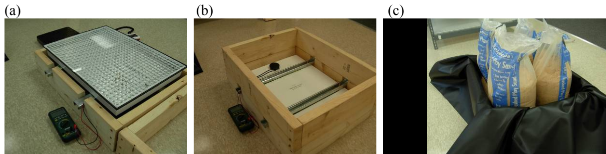
Figure 5. Mechanical loading setup for the (a) top of the module, (b) backside of the module, and (c) after covering with a tarp and four 35-lb bags of sand.
