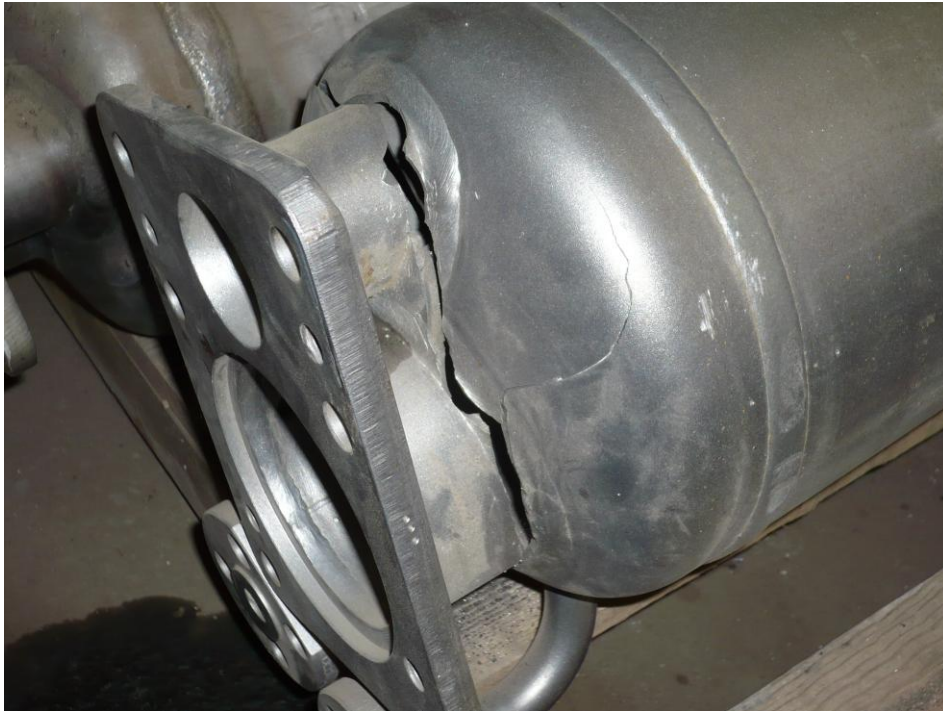
Figure 6: Column Failure due to Harmonic vibration
