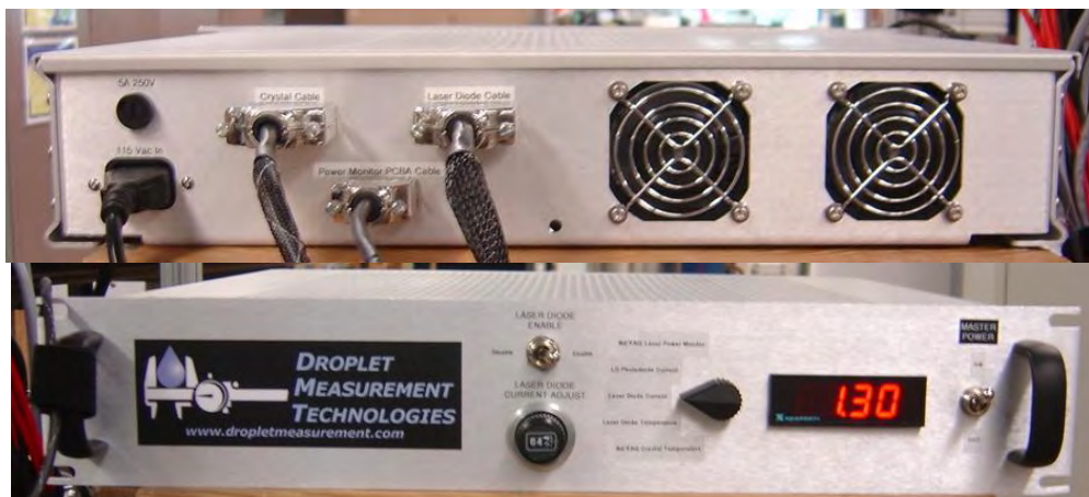
Figure 3. Pictures of the front and back of the finished electronics control box.
