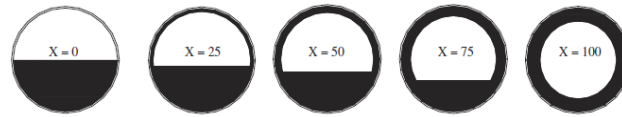
Figure 5.10 Filling profiles for UF 6 cylinders. x represents the fraction of the UF 6 that adheres to the walls before gravitational filling causes the remainder to fill the bottom of the cylinder.
