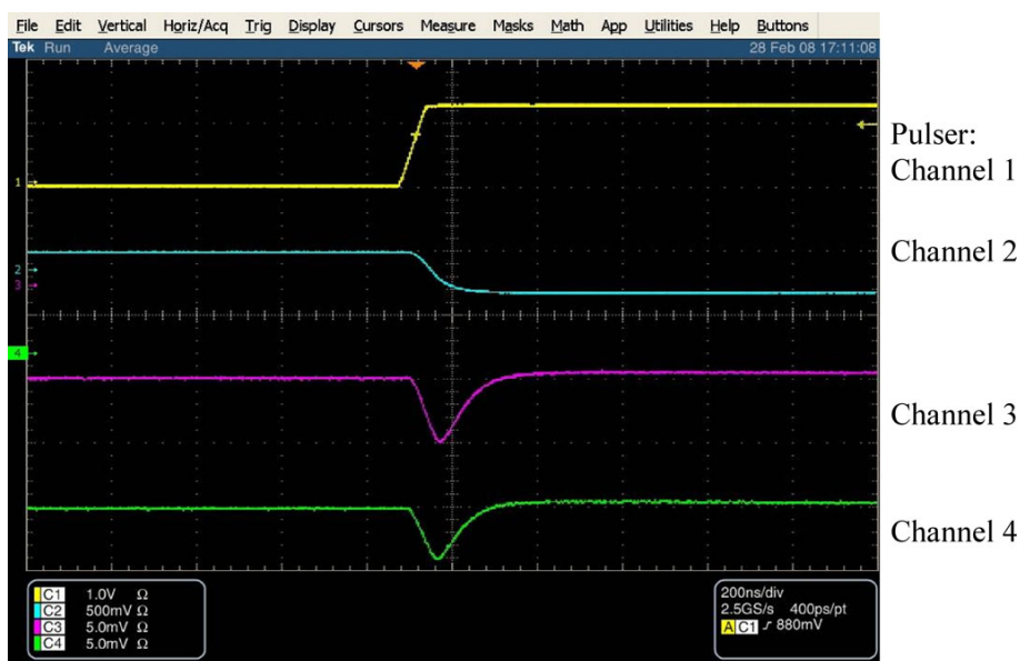
Figure 9: Scope traces of sample signal crosstalk.
