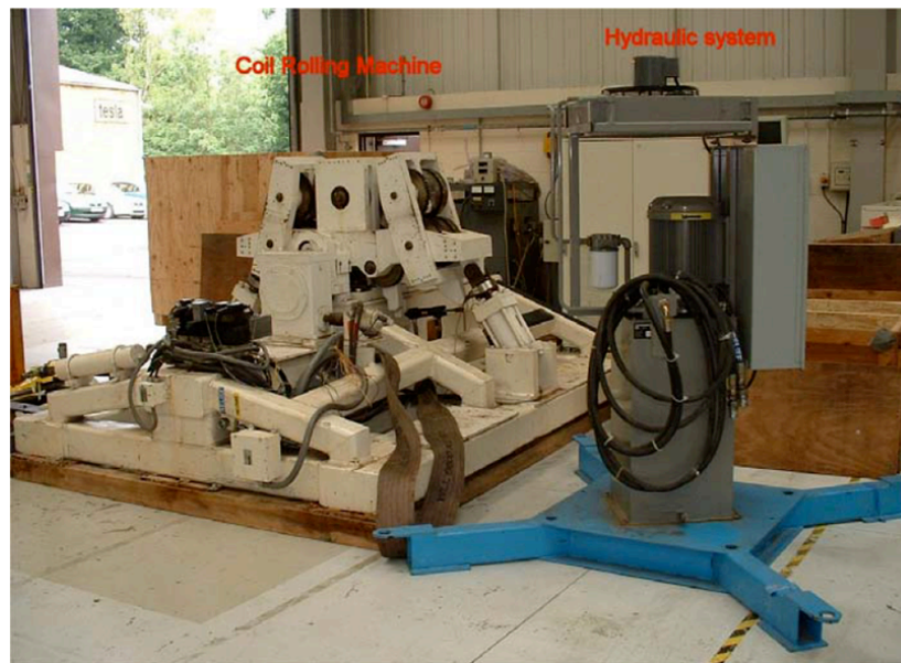
Fig. 10. Coil rolling machine and hydraulic system.
