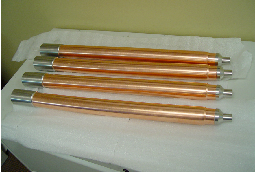
Fig. 25. CSI electric terminals received after brazing.
