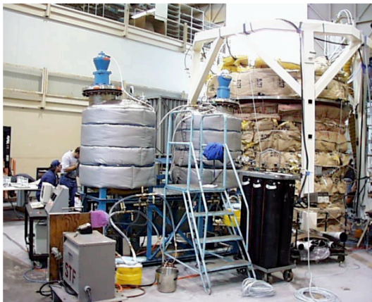
(a) Mixing System With Two Tanks
