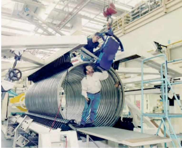
Fig. 11. Three-point bender used to straighten the rolled conductor.
