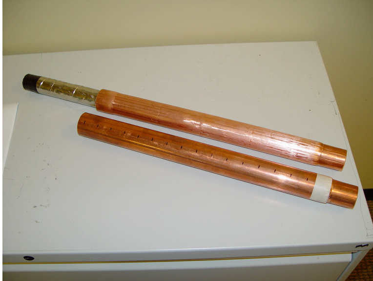
Fig. 27. Compaction test results. Tubes before and after compaction.
