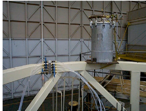
(b) VPI Resin Exit Tubing on Top of Magnet (c) VPI Vacuum Tank Above Magnet
