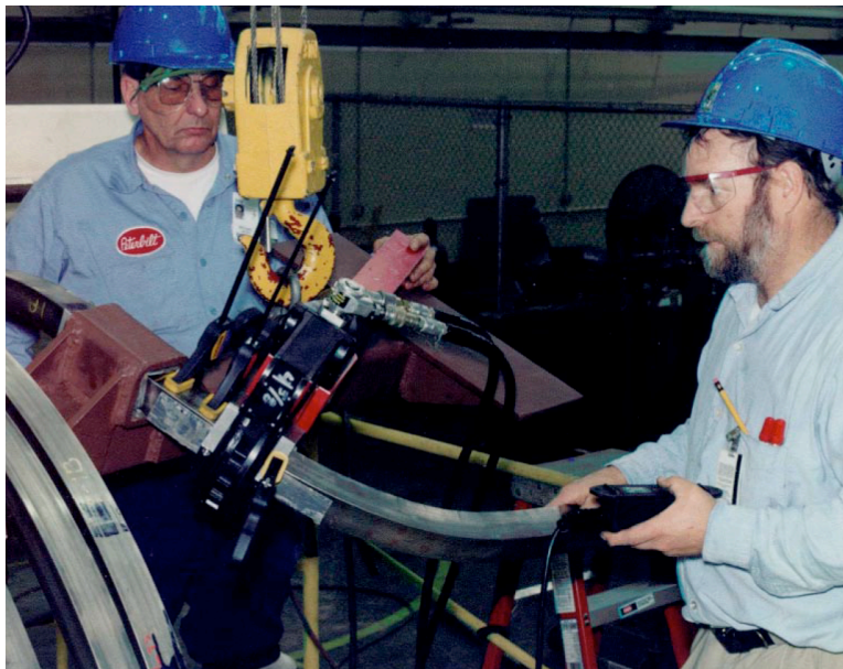
Fig. 14. Twisting tool used to form the lead.
