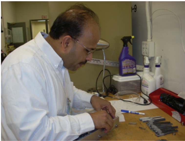
Umesh Gandhi, Toyota Research Institute, prepares a tensile sample for high strain rate tensile testing with digital image correlation.
