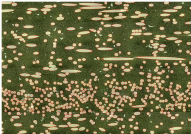
Cross section of material showing discontinuous glass fibers in quasi-random orientation (diameter 15 \mu\text{m} ).
