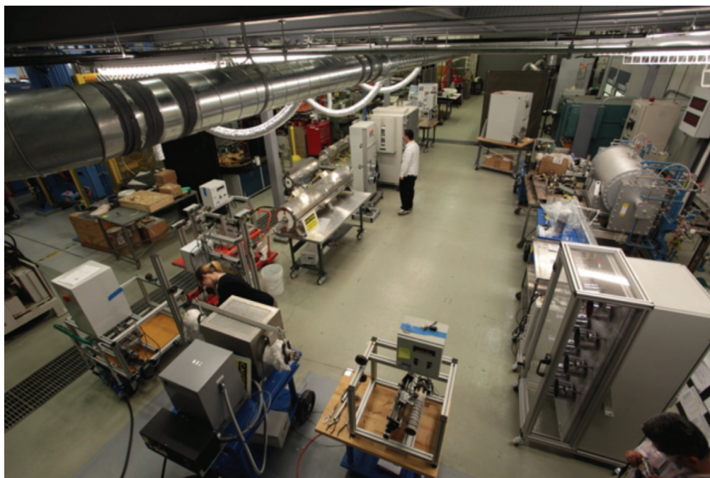
ORNL's highly versatile, modular precursor and fiber evaluation system capable of processing fibers in tow counts from 20 to more than 50,000 filaments.
