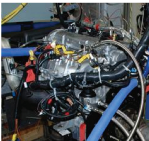
Four-cylinder research engine modified from a production engine by Delphi.
