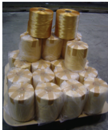
Textile tow precursor as produced by FISIFE and supplied to ORNL on spools for evaluation. Note the golden color of this precursor fiber, which is indicative of the specialized pretreatment that was developed and implemented by ORNL and FISIFE.
