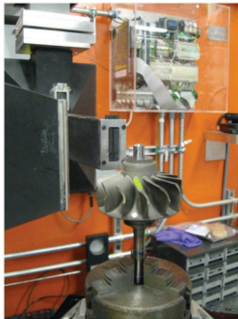
Honeywell SWA mounted on the NRSF2 beam line sample stage.
