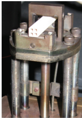
Experimental set up for measuring elastic modulus. The 2 × 2 cell specimen is loaded in 3-point-bending apparatus, and its deflection response is measured as a function of frequency while oscillation amplitude is held constant.
