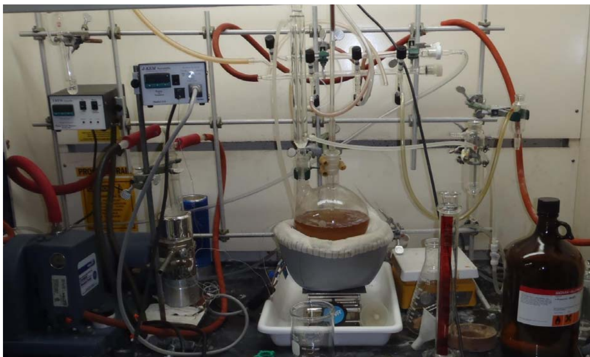
Fig. 5. Synthesis of a several hundred mL batch of 1-phenylnaphthalene in a chemical fume hood.
