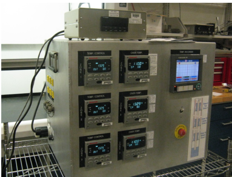
Fig. 9. PID controller for heater element inserted into the copper block. Channels were also used to monitor and record the temperatures in the inner and outer blocks. One channel was used for control, and three were used to monitor temperatures in the block.
