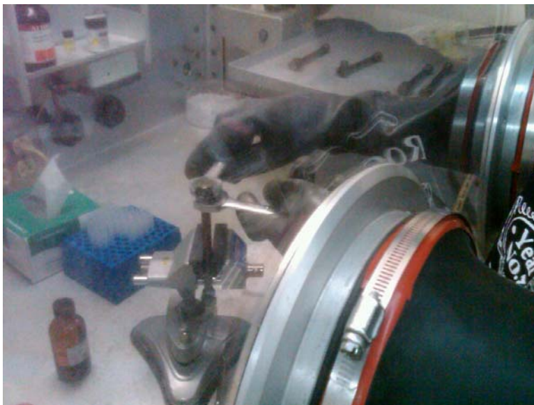
Fig. 8. Capping of the fluid sample holder in the dry box under an argon atmosphere.
