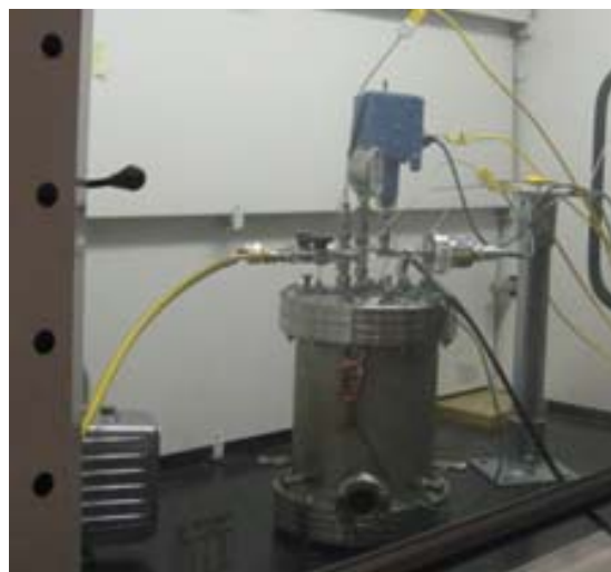
Fig. 7. Furnace assembly in evacuated shroud. The shroud could also be pressurized with gas to increase convective heat transfer.
