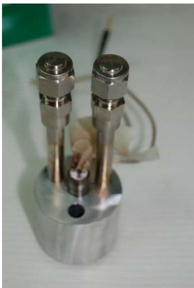
Fig. 13. Aluminum cell used for ramping experiments, showing two sample holders and embedded heater.
