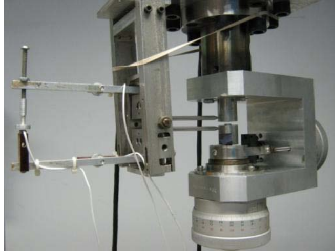
Figure 8. Calibration of the biaxial extensometer.
