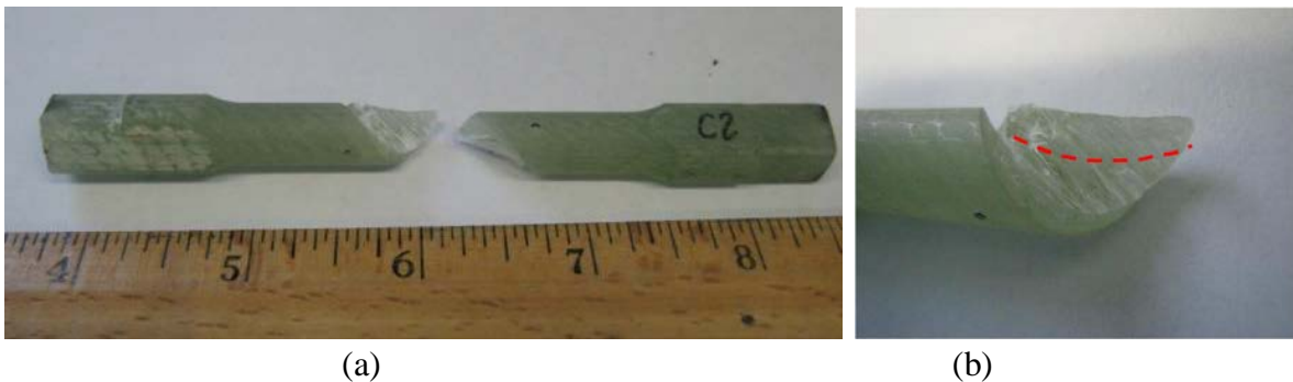
Figure 50. Pictures of a failed C-type sample (#C-2).
