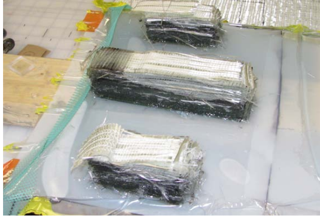
Figure 21. Failed first attempt of sandwich specimen.
