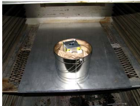
Figure 16. The resin-filled mold in a convection oven.
