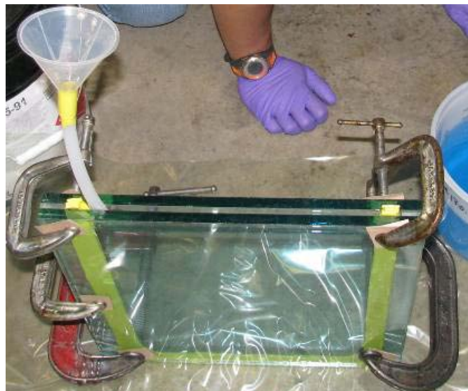
Figure 4. Parallel glass-plate mold for the flat neat-resin laminate
