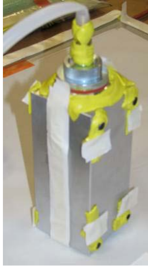
Figure 12. Sealing the mold to prevent leaks prior to pouring.
