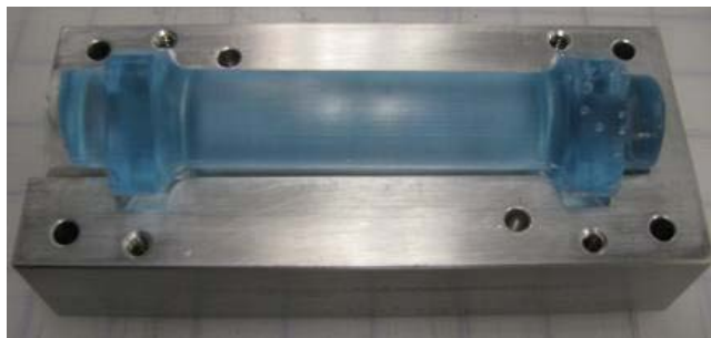
Figure 11. Half of the mold with demolded neat resin.
