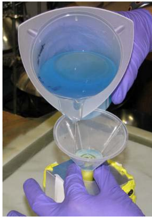
Figure 13. Careful pouring of the resin on the conical wall of the funnel.
