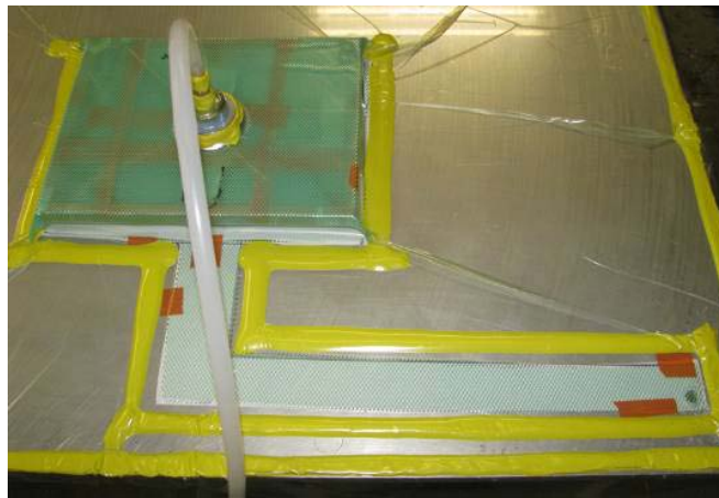
Figure 19. First attempt to manufacture sandwich test specimen.
