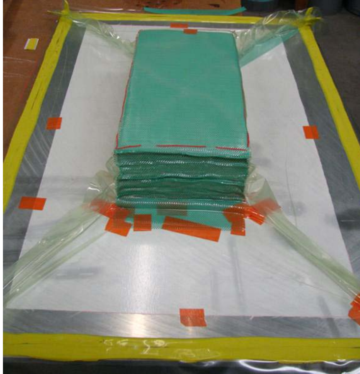
Figure 23. Infusion setup for 4"-thick composite laminate.
