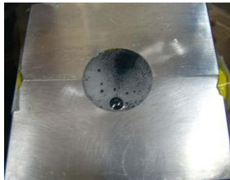
Figure 15. Second degassing after pouring for SNTT with tackified fabric.
