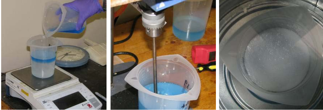
Figure 3. Weighing, mixing and degassing of resin mix.
