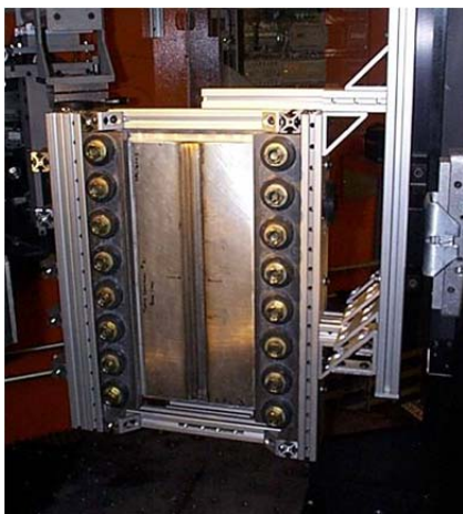
Figure 1. A Plate is mounted within a frame built with 80/20 – notice the hardware is in the plane of the plate. The frame readily is attached to the SPS.
