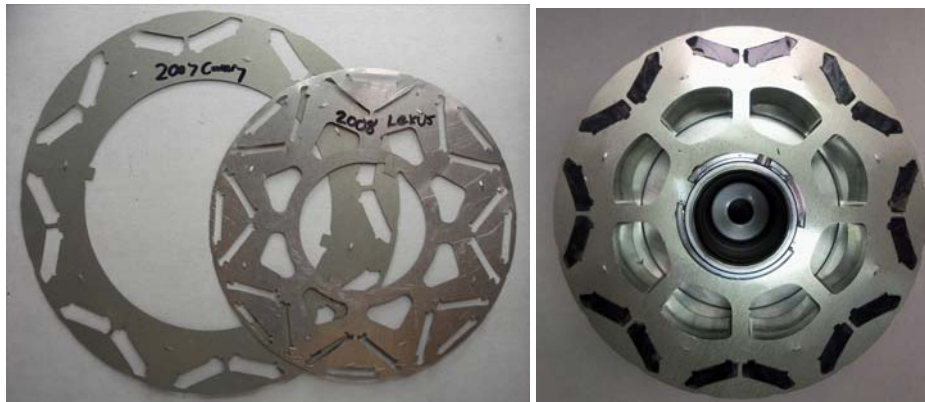
Fig. 2.63. Comparison of motor rotor laminations, Camry (left), LS 600h (middle), and 2010 Prius (right).
