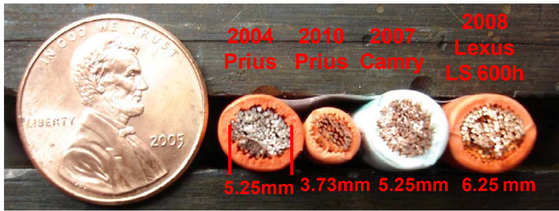
Fig. 2.61. Comparison of motor conductors between PCU and ECVT.
