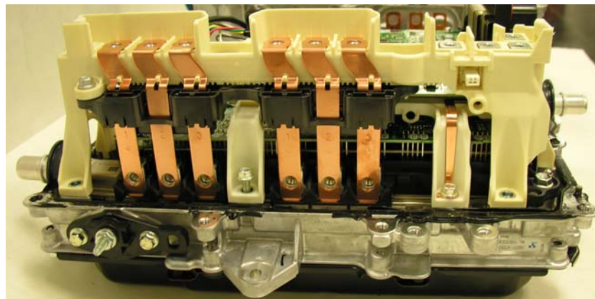
Fig. 2.8. DC, motor, and generator connection terminals.
