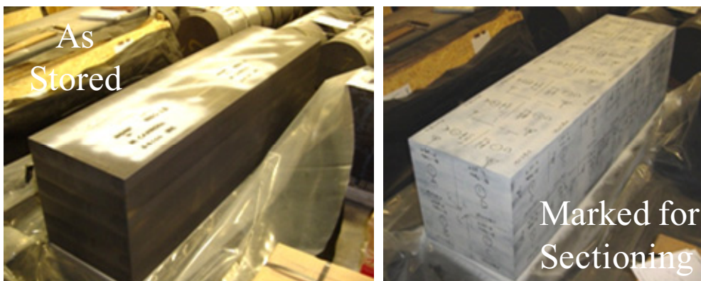
Figure 4. Quality-accepted billets of nuclear-grade graphite pre-labeled by project personnel prior to sectioning in order to ensure traceability of individual locations.
