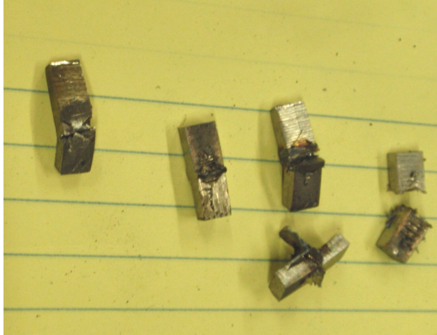
Figure 32. Small pieces before and after bending
