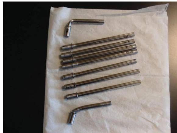
Figure 43. Lack of consistency in welded samples
