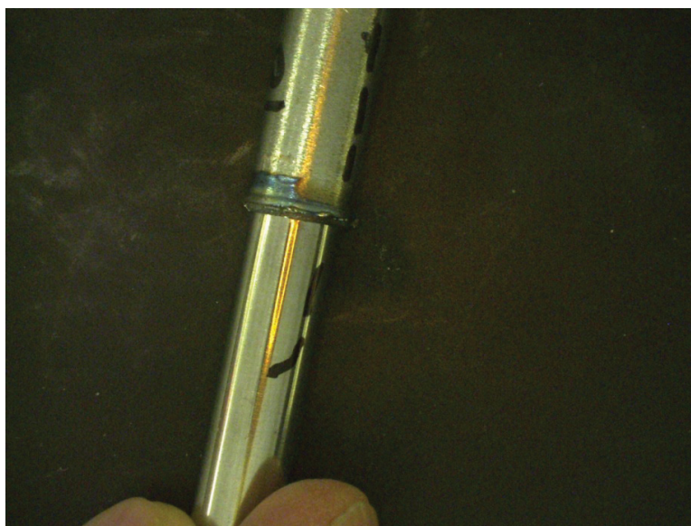
Figure 38. Uneven heating or tempering mark on half of end plug.
