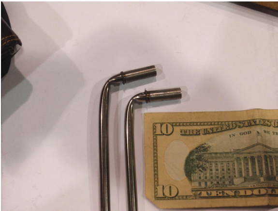
Figure 3. Weld stressing, bent cladding
