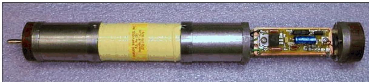
Figure 2. Oil-well logging device that utilized  $^{241}\text{Am}$ .
