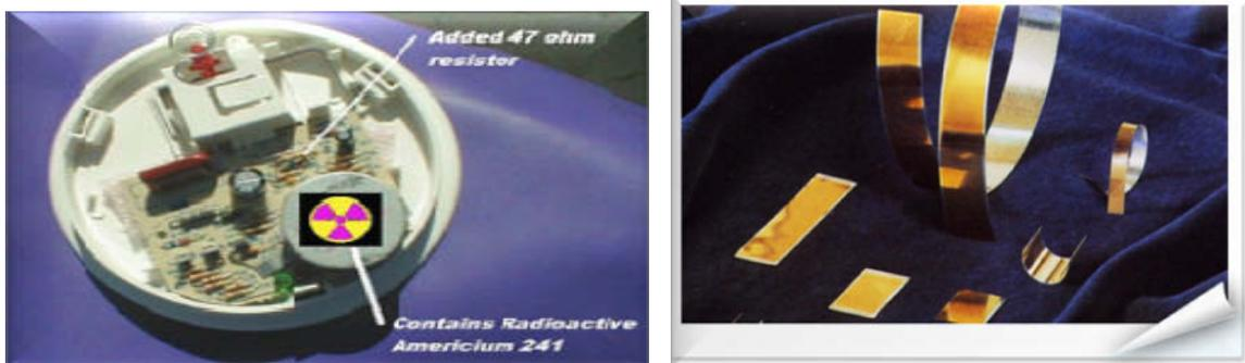
Figure 1. Smoke detectors (left) employ  $^{241}\text{Am}$  foil (right) as an alpha source.
