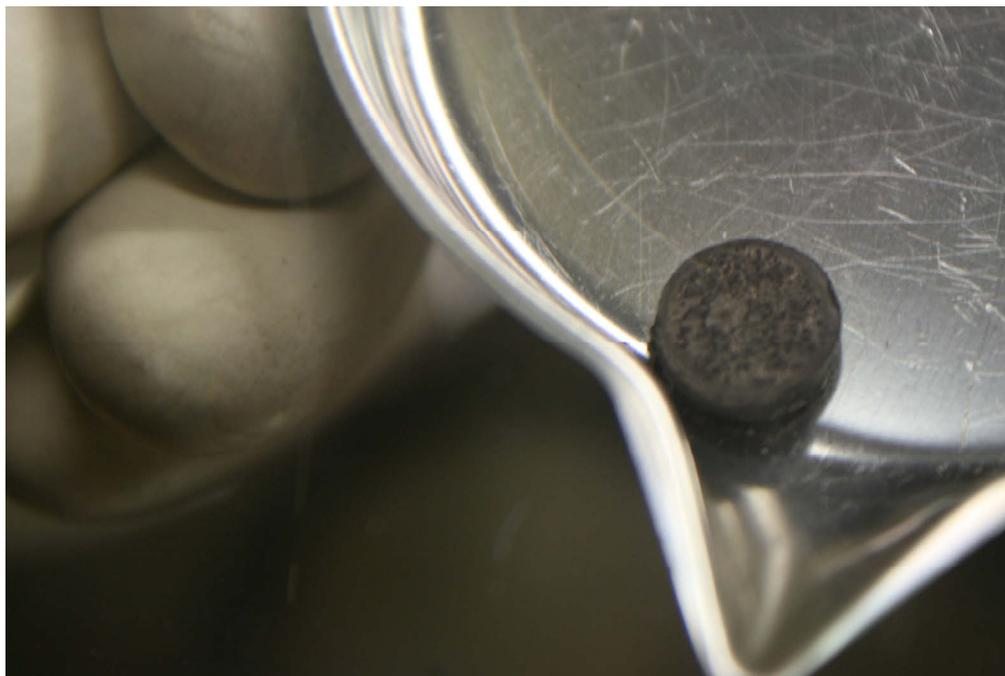
Figure 6. Pellet containing La-metal plus oxides after exposure to high temperature.
