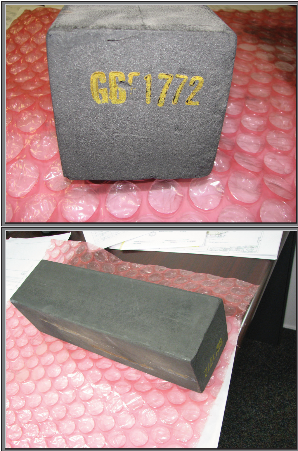
Figure 1.39. Unfinished Graphite Reflector Block.
