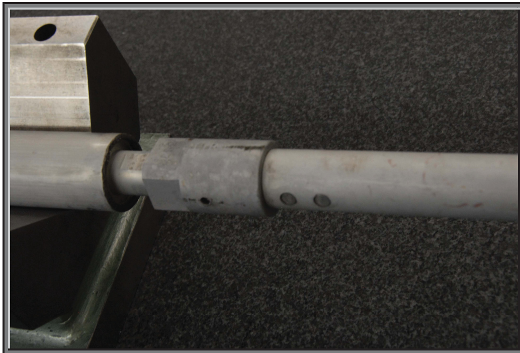
Figure 1.34. Interface between Control Rod and Extension Rod.
