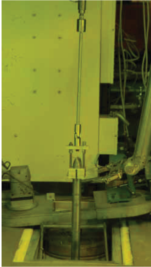
Figure 6. Test train holder (shown in the boxed region) used to mount the test train in the HFEF PGS positioning stage.
