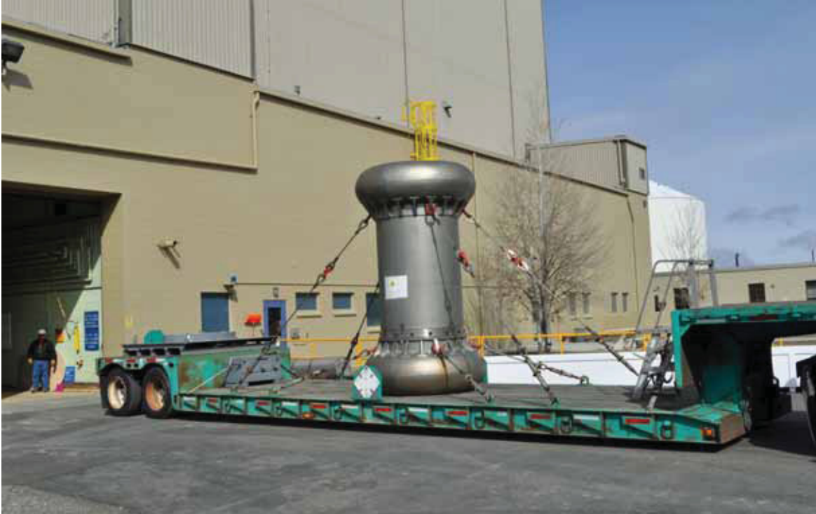
Figure 3. GE-2000 shipping cask with AGR-1 test train backing into the HFEF facility for unloading.
