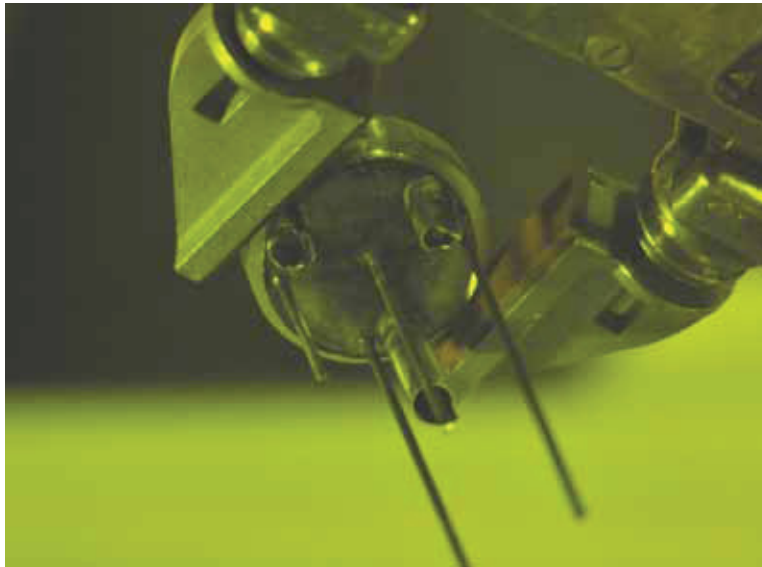
Figure 21. Through-tubes of Capsule 4 that broke near the capsule head.
