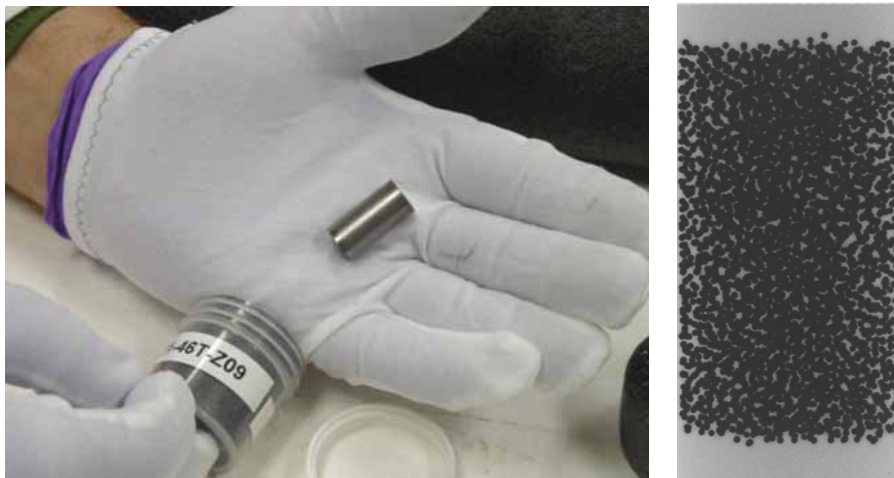
Figure 1. Photograph (left) and x-radiograph (right) of an unirradiated baseline AGR-1 fuel compact. Uranium oxycarbide kernels and nonfueled end caps are clearly visible in the x-radiograph.
