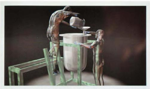
1 Working conditions at the time of the accident. Ouchi was supporting the funnel used to pour the uranium solution. Masato Shinohara, who was pouring the solution, was also exposed to a high dose of neutron beam radiation.
