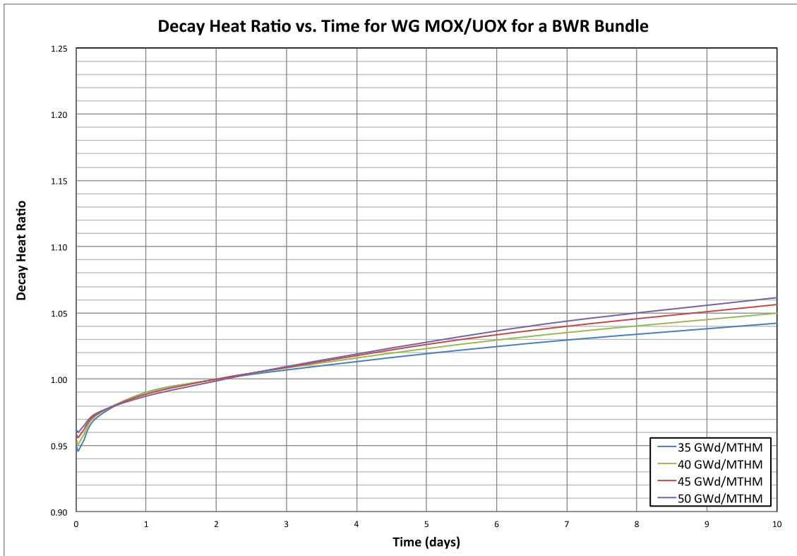
Fig. 18. Decay heat ratio as a function of time for WG-MOX for the first 10 days after discharge (BWR).
