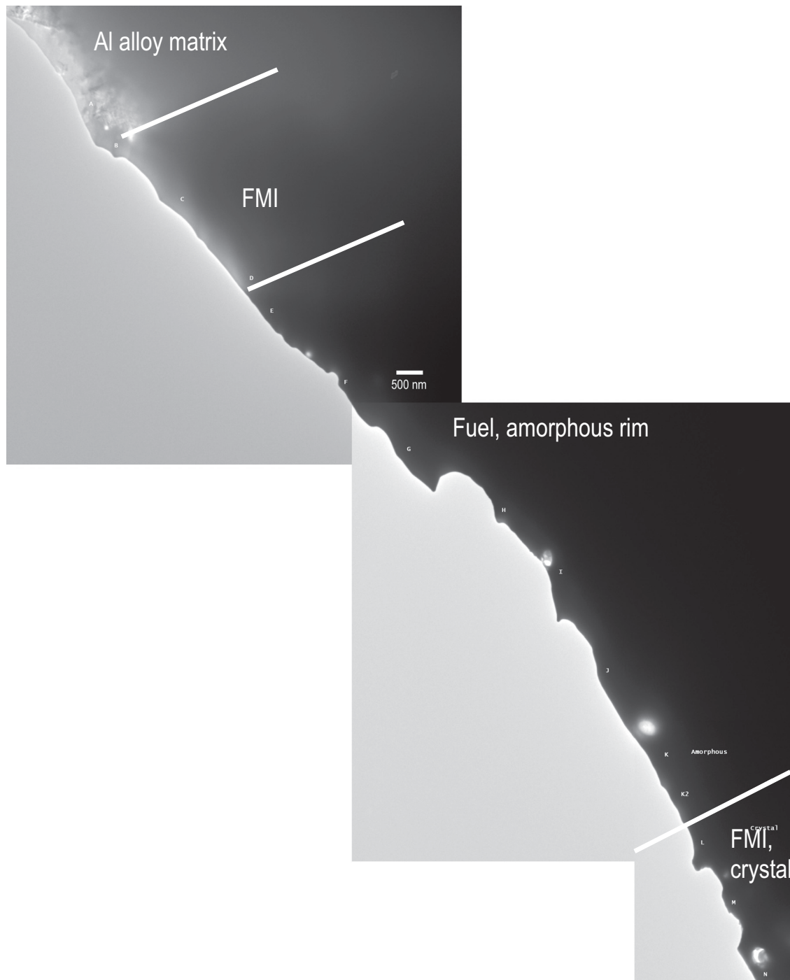
Figure 4.66: Montage of BF TEM images showing a typical amorphous rim microstructure in RERTR-7 H.Flux.
