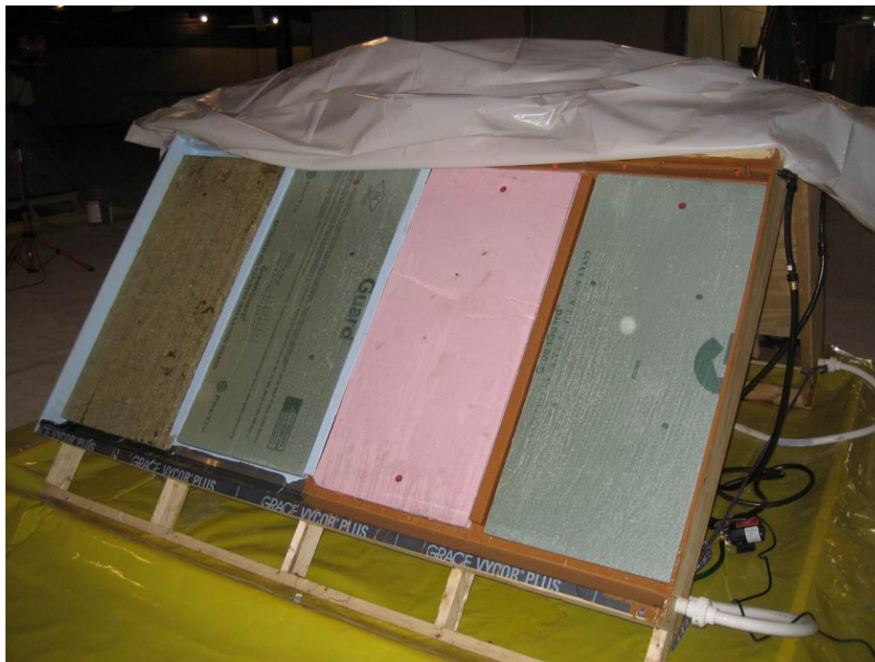
Figure 18. Drainage testing durability spray rack
