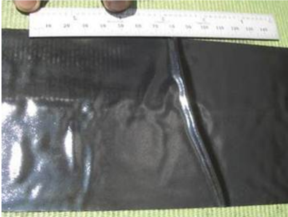
Figure 9. Wrinkle caused by thermal cycling and expansion/contraction
