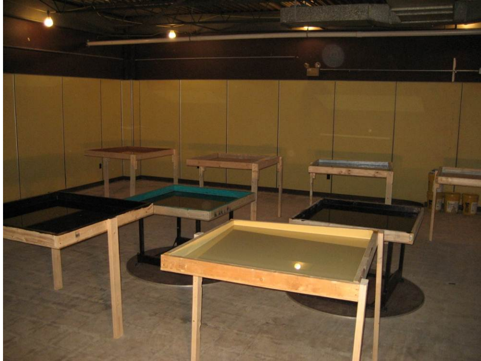
Figure 15. Liquid applied membrane water baths
