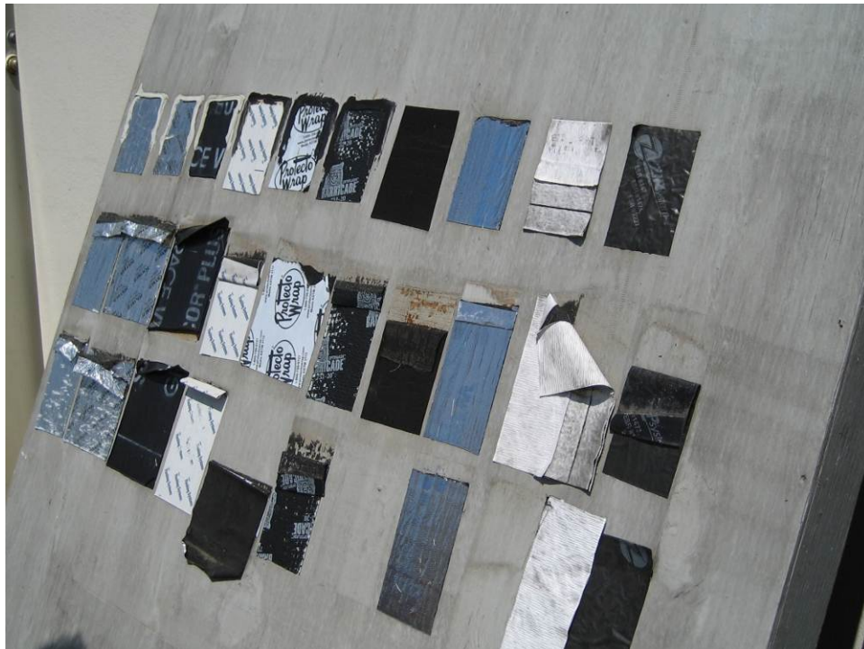
Figure 21. Exposure testing of peel and stick membranes
