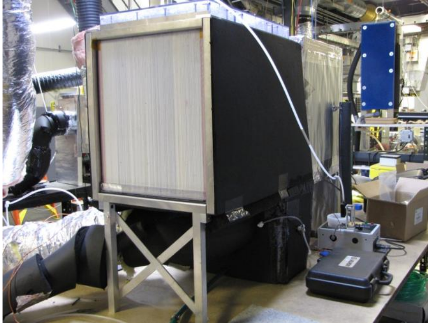
Figure 2–7 Fully assembled view of ALL Research second-stage conditioner (outlet airstream 2 shown)
