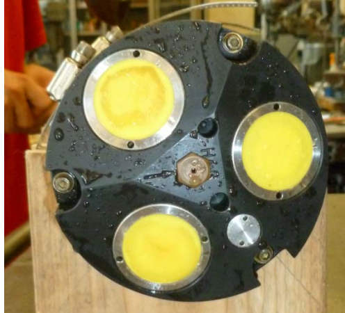
Figure 3.6 The SonTek ADP used in the experiment.
