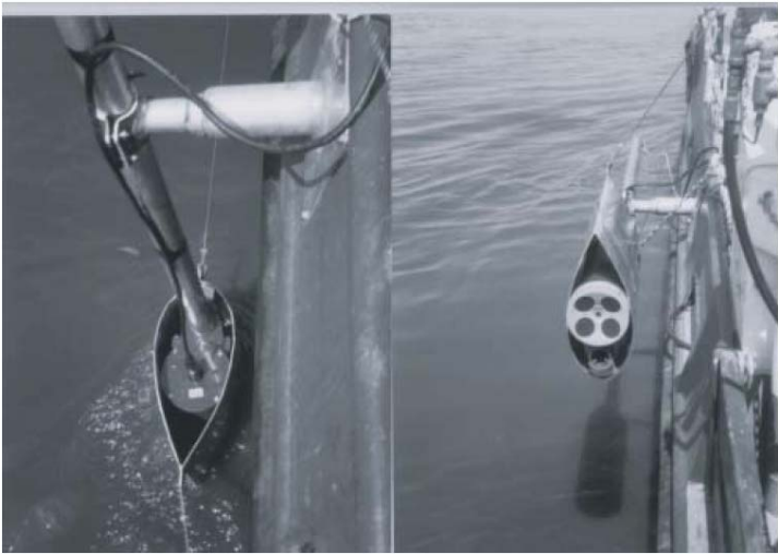
Figure 2.13 Two views of shipboard ADCP side-swing mount on a 30-meter (95-foot) vessel (Simpson 2001).
