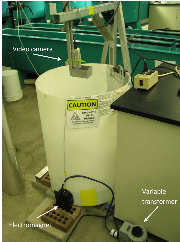
Figure 6. Experimental tank used to test the response of fish to variable magnetic fields created by an AC electromagnet.
