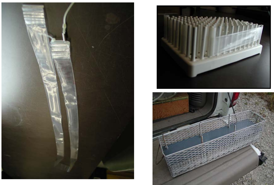
Fig. 5. Semi-permeable membrane devices (SPMDs) are comprised of polyethylene tubes containing a layer of triolein oil (left) and are deployed by wrapping around a test tube rack and caged to help prevent damage from debris or biota during deployment (right, top and bottom). Various cage setups are used depending on whether deployed at a stream or storm drain site.
