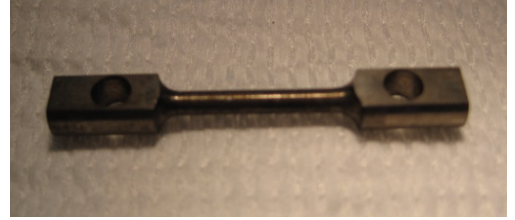
Figure 3: Sample with small fixture hole (at the left) comparing to the normal (expected) hole diameter.
