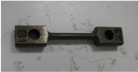
Figure 4: Deep coarse numbering: the coarse number of specimen (at the left) and unexpected undocumented characters (at the right).
