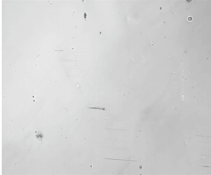
Figure 5: Sample B123 surface (one of samples' heads). A clear surface with some insignificant amount of carbides and other inclusions is observed. Very light scratches are also visible. Sample handling caused the minor scratches on the heads.
